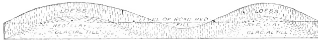
FIGURE 2.—Sketch profile showing relation of loess to underlying beds of clay and glacial till in railroad cuts west of Omaha, Nebr.
